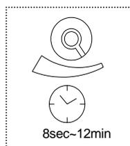
The light can be set to stay ON for any period of time between approx. 8sec(turn fully anticlockwise) and a maximum of 12min(turn fully clockwise). Any movement detected before this time elapse will re-start the timer. It is recommended to select the shortest time for adjusting the
