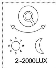
The chosen light response threshold can be infinitely from approx. 2-2000lux. Turn it fully anti-clockwise to select dusk- to-dawn operation at about 2 lux. Turn it fully clockwise to select daylight operation at about 2000lux. The knob must be turned fully clockwise when adjusting the detection zone and performing the walk test in daylight.
