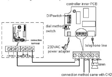
4. Connect power adapter: the adapter requires: input 230VAC, output 12VDC, and current ≥1000mA. During AC power is on, standby battery will be charged automatically. When AC power cut off, the product works by standby battery entirely. Under the condition that AC power cut off and the standby battery is charged entirely, the battery's static waiting time is 8 hours.
